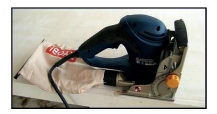
The image on the previous page is the Ryobi biscuit joiner with the fence recessed. The image below is of the Ryobi biscuit joiner with the fence set to control the location of the biscuit joint to be cut on the material.
